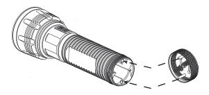
Inserting batteries in a dark environment: Two of the four battery slots in the EA81's battery compartment feature grooves indicating that batteries should be inserted with the negative (-) ends facing forward, while the two slots with no grooves require the batteries to be inserted with the positive (+) ends facing forward. In this way, batteries can be inserted correctly through tactile feedback alone.
