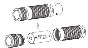
Always ensure batteries are inserted with the positive (+) ends pointing toward the flashlight head. If incorrectly installed, the flashlight will not work.
